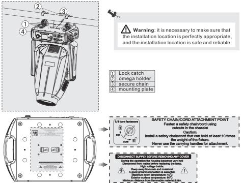
According to the four screws broke open the back cover, back cover marked as shown direction turn to change the bulb to corresponding card slot can be removed. According to the chart Three screws rotating back cover, can adjust the bulb location. As shown in figure;
